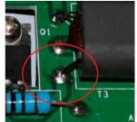
5. Open one side of the T3 transformer (The red circle shown the graphic below), and then connect the multimeter/ammeter between the pads for L1; make sure meter is at 10A range position. Adjust the potentiometer RV2 slowly anti-clockwise until the measured current is between 25 and 30mA. Make sure ammeter leads do not pass close to the input side of the board. (See my note below on using a resistor and voltmeter instead
