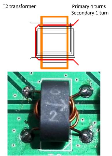
You will note that the schematic shows the multiple turn winding and the pads numbered one and two towards the IRF530 gates while the photos show a directional arrow to the right. The illustration above shows one turn to the right (IRF530 gates). I reasoned that the IRF530 gates are the low impedance side so I put the single turn winding to drive the gates.
